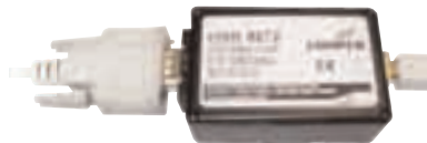
RS232 to USB - Wireless panel to PC (site installer)
