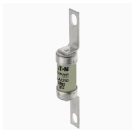
Fuse-link, LV, 10 A, AC 550 V, BS88/A2, 14 x 85 mm, gL/gG, BS
